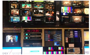
To keep up with our growing business from sports and corporate clients, we have added eight Ericsson RX 8200 receivers and two AVP 3000 encoders to our inventory. We have also added a third quality control (QC) station equipped with QC monitoring; a two-channel scope for waveform, vectorscope and audio monitoring; and three DekTec stream analyzers to monitor incoming and outgoing signals. Like our other QC stations, it also features ASI and SDI panels from the Trinix 512 router for QC routing.
